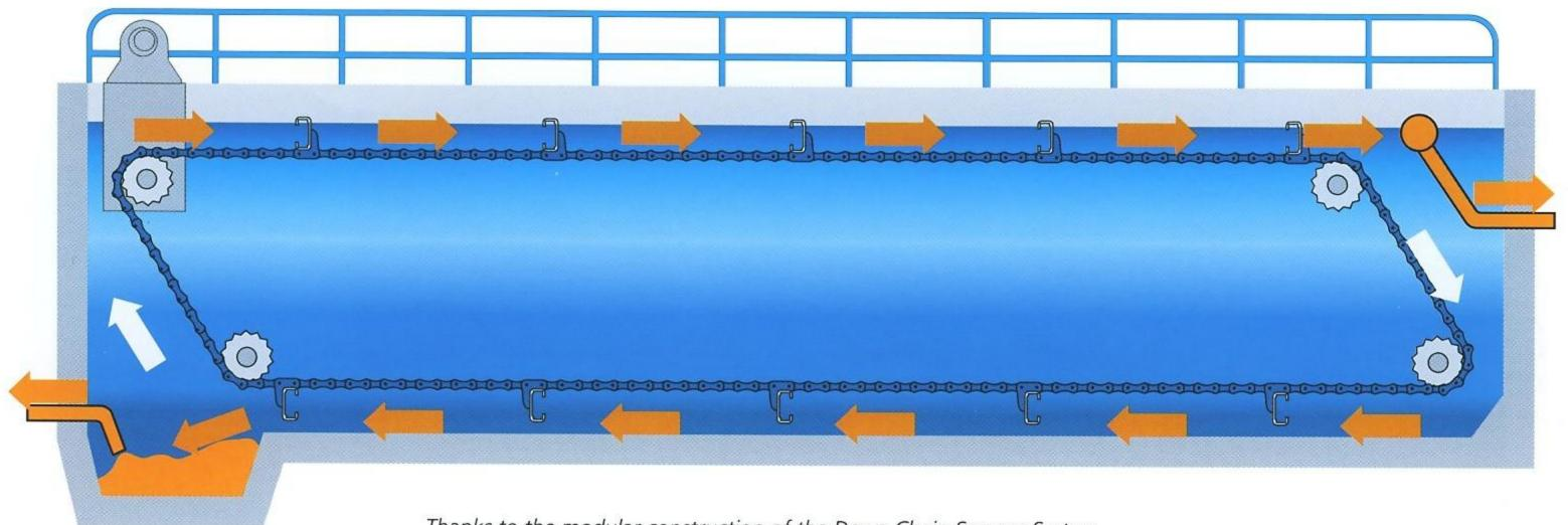
Thanks to the modular construction of the Dewa Chain Scraper System it can be easily fitted to any type of rectangular sedimentation tank.
